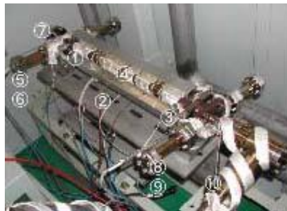
Fig. 28 Heater setup for baking at KEK.
