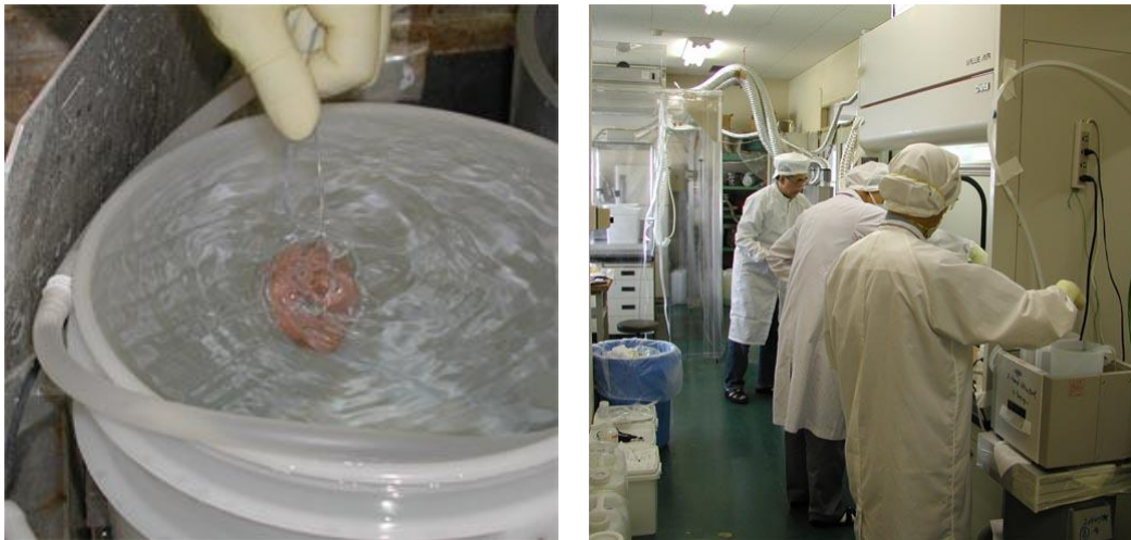
Fig. 11 Chemical rinsing process at KEK.
