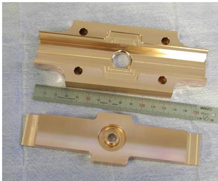
Fig. 10 Coupler parts, body (Up) and plate (Down).
